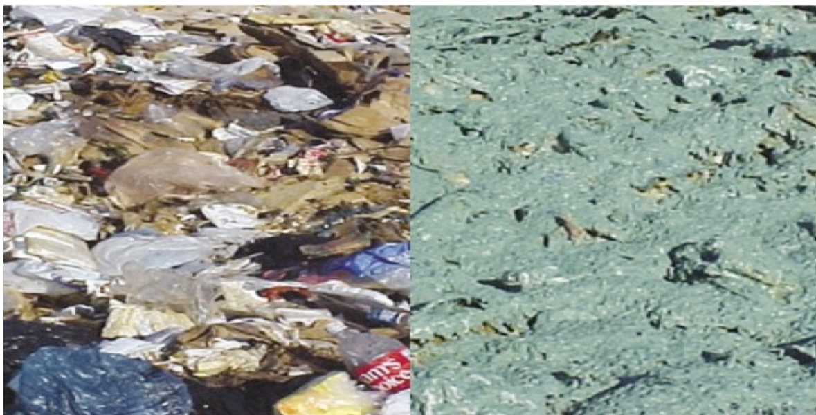
Fig. 28. The waste surface without cover (left) and with the cover (right)
