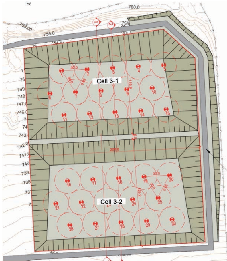
Fig. 20. Vertical gas collecting wells mounted on the III cell under the existing project
