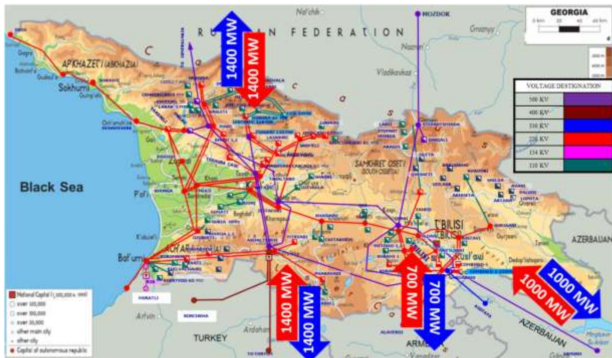
Fig. 1.16 Cross-border transfer capacities between power systems of Georgia and its neighbouring countries as for 2027
