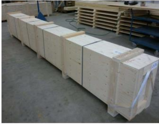
5) Picture: Antenna accessories. This box is equipped with pulling strap to make unloading from sea container easier.
