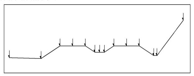
In case of sediments: the concrete lining surface is the elevation to be obtained. The thickness of sediment must be noted for each point where it is present. (In earth canals the mirror pole must be placed gently (without pressure or dropping it) on the existing sediment)
