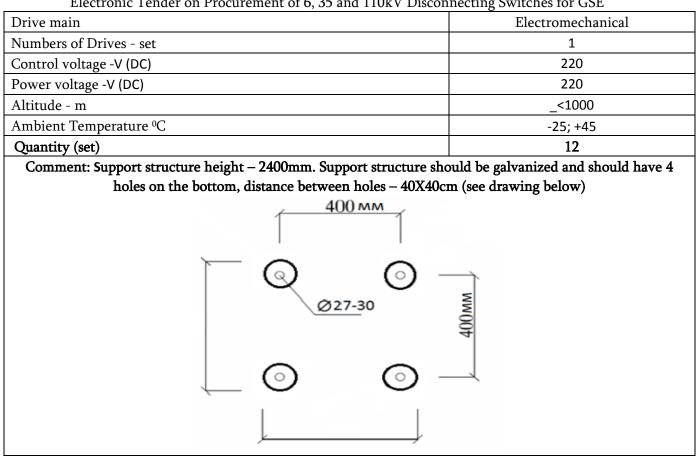
Electronic Tender on Procurement of 6, 35 and 110kV Disconnecting Switches for GSE
