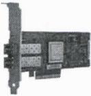
2 x HPE StoreFabric 16Gb Dual Port Fibre Channel Host Bus Adapter
